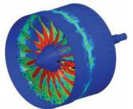
The remaining half of the quadcopter is ingested and is struck by a second blade; stress increases as parts of the blade hit the casing; loss of blade mass exacerbates the imbalance and stress.
