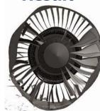
The titanium-alloy casing is significantly deformed.
