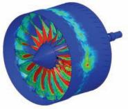
Damage spreads to a third blade; the imbalance worsens; pieces of the drone are now impacting the casing.
