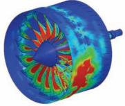
The quadcopter is obliterated; three fan blades are catastrophically damaged; the remaining blades contact the casing; stress grows, shown in red, but the casing holds.
